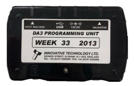
Once the files are loaded onto the DA3, the validator can be updated. Simply remove the host machine cable and plug this into the "Host machine" port on the DA3 as shown in the image above. You will then need a ribbon cable to connect the DA3 to the validator itself, via the "validator" port. The DA3 should now be sat in-line between host and validator, with the DA3 being powered from the host connector.
