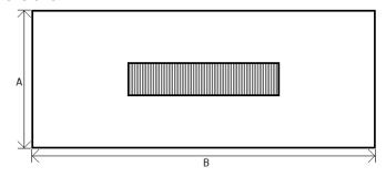
Tickets should have a width (A) of 65mm to 82mm, the smaller the ticket the larger barcode width should be used.
