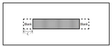
A blank space (C) is required on either side of the barcode as pictures or text may be seen as part of the barcode value.
