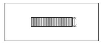
The barcode itself should be no thinner (E) than 10mm. The narrow bar width between 0.5mm and 0.6mm, with the wide narrow ratio (W:N) being 2:1.
